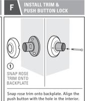
push button with the hole in the interior. Thread the button into the housing.
